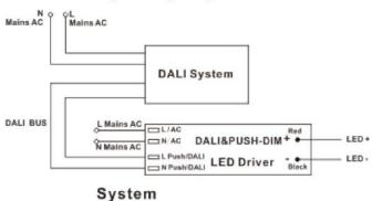
Push-Dimming Wiring Diagram2
