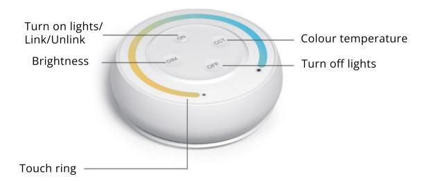
**Touch ring:** Adjusts both colour temperature and brightness. Use the DIM or CCT button to select which one you're adjusting. By default, if the remote is not operated for 3 seconds, it will switch back to brightness mode.
