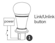
Switch off the light you want to link. Wait 10 seconds, then switch it on again. Short press the ON button 3 times within 3 seconds.
