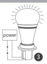
Switch off the light you want to link. Wait 10 seconds, then switch it on again. Short press the ON button 5 times within 3 seconds.
