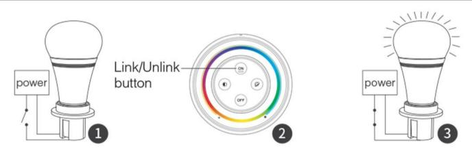
Switch off the light you want to link. Wait 10 seconds, then switch it on again. Short press the ON button 3 times within 3 seconds.
