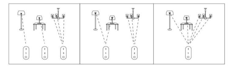
**Note:** One remote can control an unlimited number of lights and controllers, but each lamp or controller can only be controlled by a maximum of four remotes.
