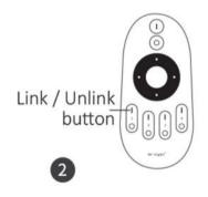
Short press the "I" button for the zone you want to link the light to 5 times within 3 seconds.
