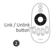
Short press the "I" button for the zone you want to link the light to 3 times within 3 seconds.
